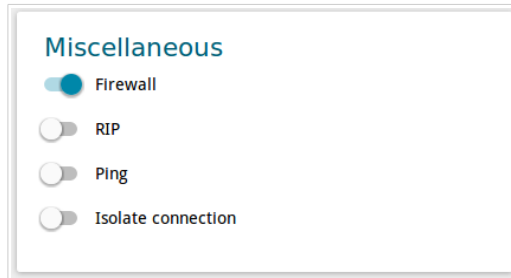
Figure 42. The page for creating a new Static IPv6 connection. The Miscellaneous section.
