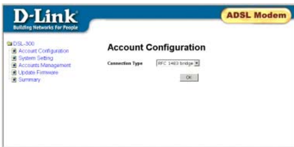
Figure 7. RFC 1483 Bridge Account Configuration
