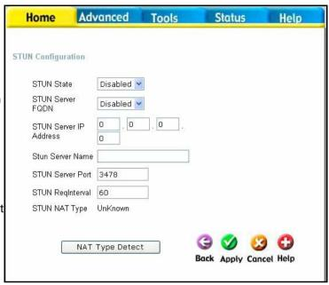
STUN is useful if you need to use the DVG-G1402S behind a modem or router that provides the connection to your ISP and then to the Internet and does not support symetric NAT. You will need access to a STUN server on the Internet and its IP address to use STUN on the DVG-G1402S.
