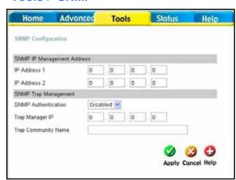
Use SNMP to configure system features for proper operation, performance monitoring, and detection of potential problems in the Router or network.
