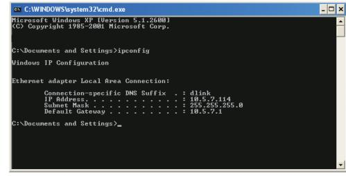
If the address is 0.0.0.0, check your adapter installation, security settings, and the settings on your router. Some firewall software programs may block a DHCP request on newly installed adapters.
