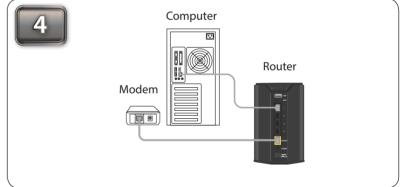
Position your router close to your modem and a computer. Unplug the Ethernet cable from your modem (or Plug one end of the included blue Ethernet cable that came with your router into the yellow port labeled **INTERNET** on the back of the router. Plug the other end of this cable into the Ethernet port on your modem.
