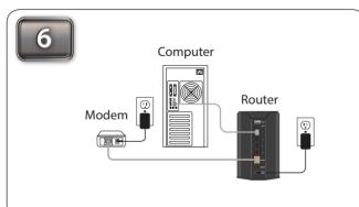
Connect the supplied power adapter into the power port on the back of the router and then plug it into a power outlet or surge protector. Press the power button and verify if the power LED is lit.
