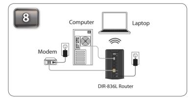
This is a sample network configuration of the setup after you have completed all the setup steps.
