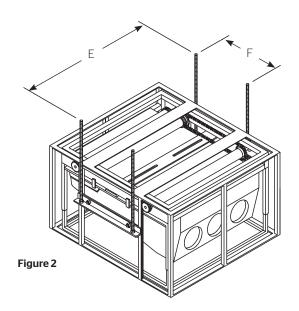
2. Mounting Da-Lift Projector Lift using 1/2" diameter threaded rods. Secure four 1/2" diameter threaded rods to the ceiling at the dimensions shown. See Figure 2, "E" and "F". Install the mounting bracket (1-1/2" x 19") to each side of Da-Lift with 1/2" diameter bolts, flat washers and nuts. Attach one nut on each rod and run the nut up to the desired height.
