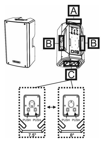
A -Upper integrated handle B - Lateral integrated handles C - Pole mount hole, with two tilt angles selection (0°/ 7.5°)
