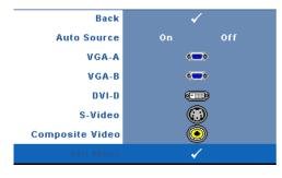
**AUTO SOURCE**—Select **On** (the default) to autodetect the available input signals. If you press the Source button when the projector is on, it automatically finds the next available input signal. Select Off to lock the current input signal. If you press the Source button when the Auto Source mode is set to Off, you can
