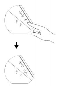
To power off the speaker, press and release the power button. The LED on the power button will fade out to indicate that the device is off.
