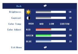
**CONTRAST**—Use ⊙ and (→ to control the degree of difference between the brightest and darkest parts of the picture. Adjusting the contrast changes the amount of black and white in the image.
