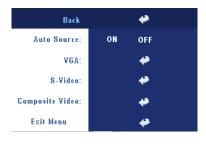
**AUTO SOURCE**—Select **ON** (the default) to autodetect the available input signals. When the projector is on and you press **SOURCE**, it automatically finds the next available input signal. Select **OFF** to lock the current input signal. When **OFF** is selected and you press **SOURCE**, you select which input signal you want to use.
