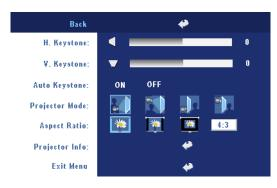
**V. KEYSTONE**—Adjust image distortion caused by tilting the projector.
