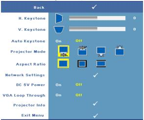
**H. KEYSTONE**—Adjusts the image distortion caused by horizontal shifting of the projector orientation.
