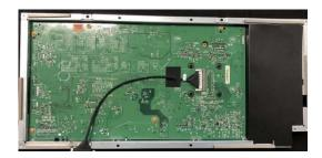
Tear off an adhesive tape from EDP cable on I/F BD
