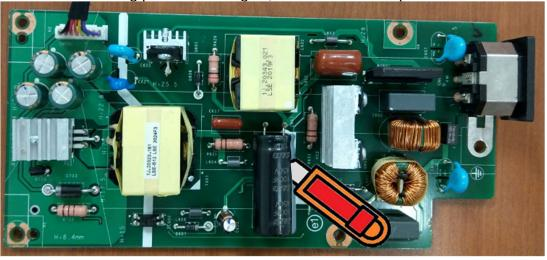
S38-3 Take out bulk cap. pin solder with soldering iron and absorber
