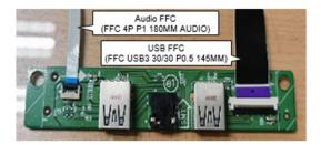
Remove FFC cable from Rear Cover, CTRL BD and CTRL+KEY BD
