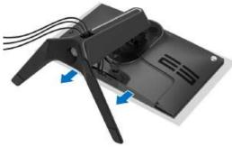
Disconnect the cables from the monitor and slide them out through the cablemanagement slot on the stand riser
