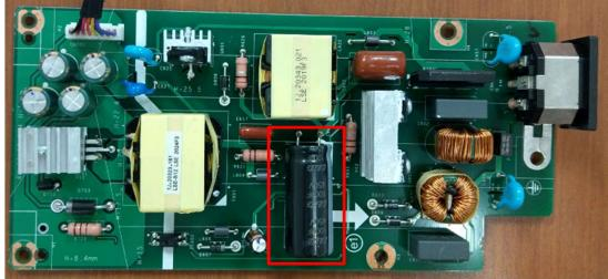
S38-1 Cut the glue between bulk cap. and PCB with a knife
