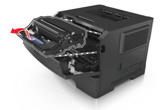
**Warning—Potential Damage:** Do not touch the shiny blue photoconductor drum under the imaging unit. Doing so may affect the quality of future print jobs.
