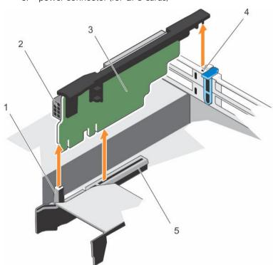
Figure 43. Removing the expansion card riser 3
