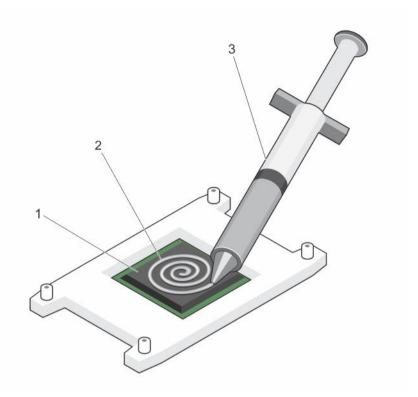
Figure 24. Applying thermal grease on the top of the processor
