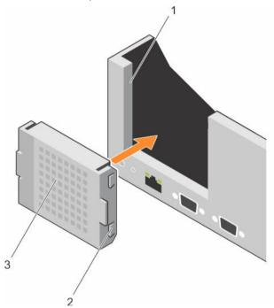
Figure 38. Installing the riser 1 blank
