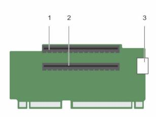
Figure 42. Identifying connectors on the expansion card riser 2
