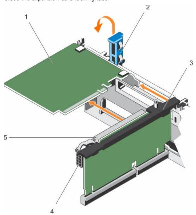
Figure 33. Removing an expansion card from expansion card riser 2 or 3
