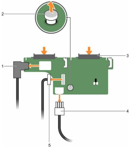
Figure 76. Removing the optional 2.5 inch (x2) hard drive backplane
