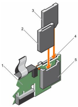
Figure 50. Installing an internal SD card
