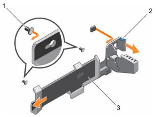
Figure 29. Removing the cable retention bracket
