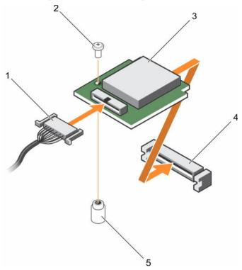
Figure 81. Installing the vFlash media unit
