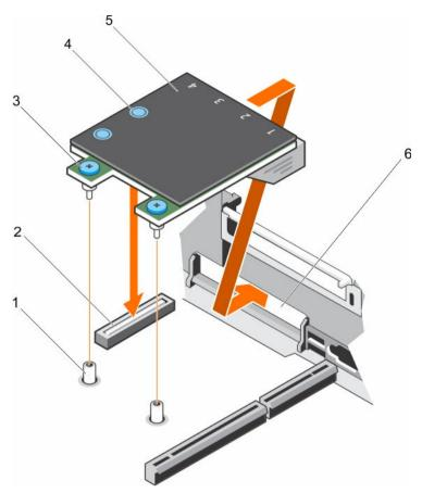
Figure 53. Installing the NDC
