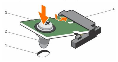
Figure 64. Installing the TPM
