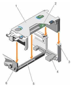
Figure 46. Installing the expansion card riser 1
