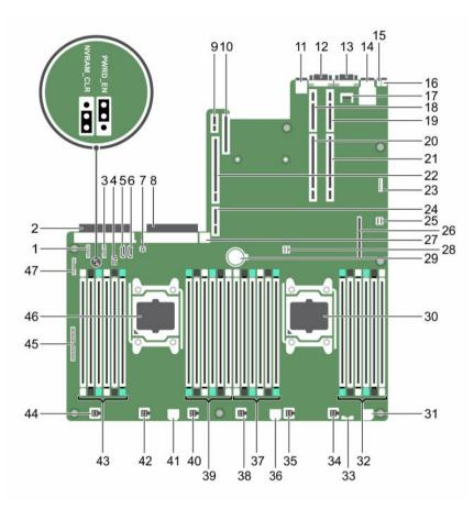
Figure 86. System board jumpers and connectors
