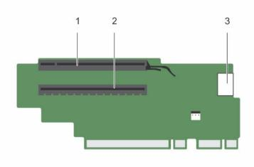
Figure 44. Identifying connectors on the expansion card riser 3 (default)
