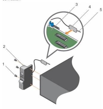
Figure 83. Installing the control panel
