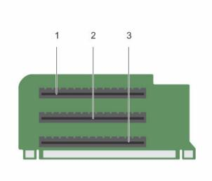
Figure 40. Identifying connectors on the expansion card riser 1
