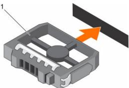
Figure 68. Installing a 3.5-inch hard drive blank
