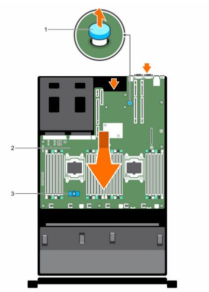
Figure 62. Removing the system board
