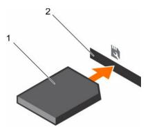
Figure 79. Installing the SD vFlash media card
