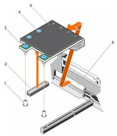
Figure 52. Removing the NDC
