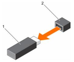
Figure 54. Removing the internal USB memory key
