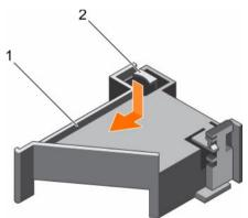
Figure 26. Installing the PCIe card holder
