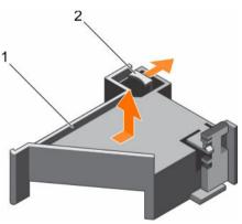
Figure 25. Removing the PCIe card holder
