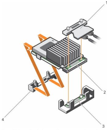
Figure 31. Removing the integrated storage controller card
