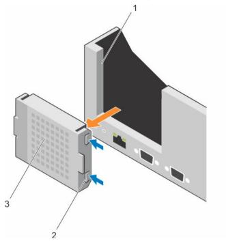
Figure 37. Removing the riser 1 blank
