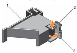
Figure 27. Opening the PCIe card holder latch
