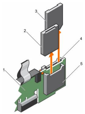
Figure 49. Removing an internal SD card
