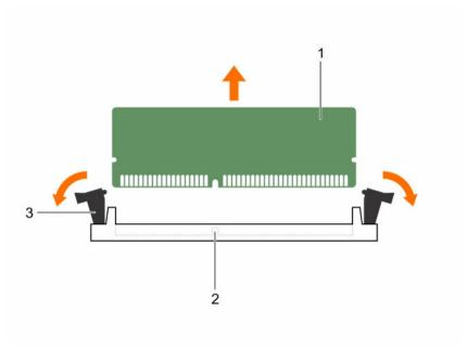
Figure 18. Removing the memory module
