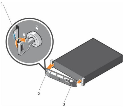
Figure 10. Removing the optional Quick Sync front bezel
