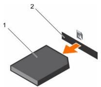
Figure 78. Removing the SD vFlash media card
