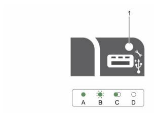
Figure 6. iDRAC Direct LED indicator
