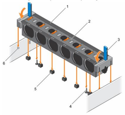
Figure 16. Installing the cooling fan assembly
