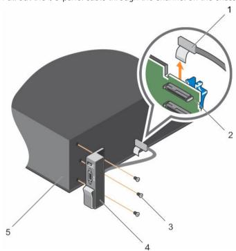
Figure 84. Removing the I/O panel
