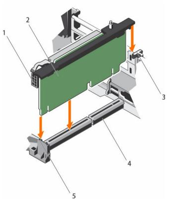
Figure 47. Installing the expansion card riser 2
