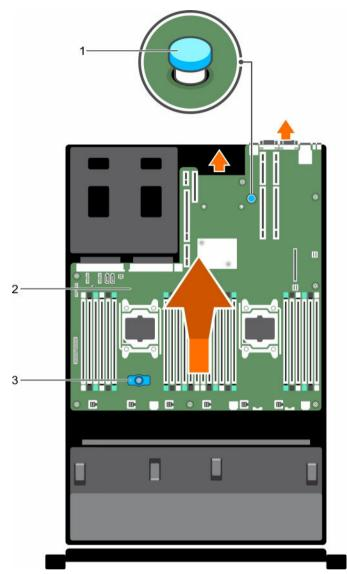
Figure 63. Installing the system board
