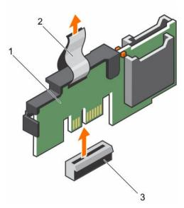
Figure 51. Removing the internal dual SD module (IDSDM)
