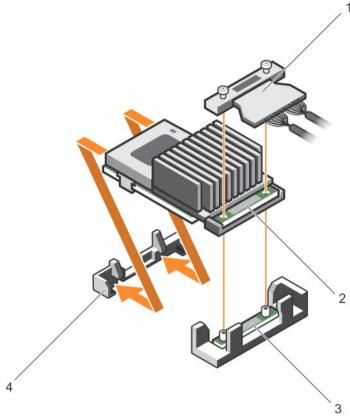
Figure 32. Installing the integrated storage controller card
