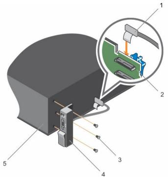
Figure 85. Installing the I/O panel
