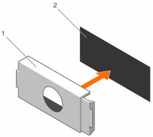
Figure 59. Installing the PSU blank
