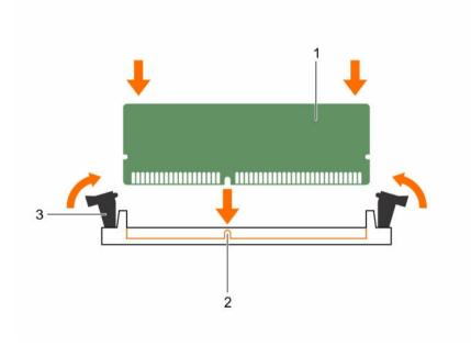
Figure 19. Installing the memory module
