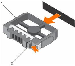
Figure 67. Removing a 3.5-inch hard drive blank
