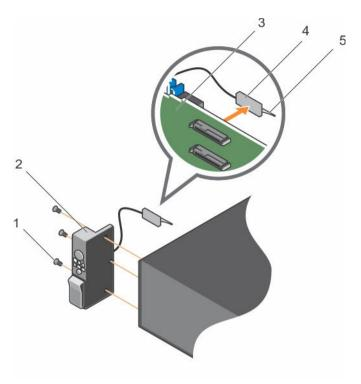
Figure 82. Removing the control panel
