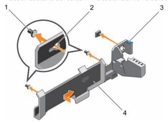
Figure 30. Installing the cable retention bracket
