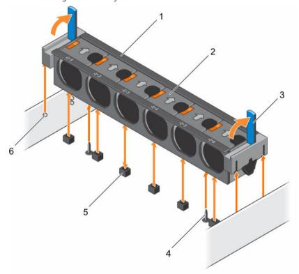
Figure 15. Removing the cooling fan assembly
