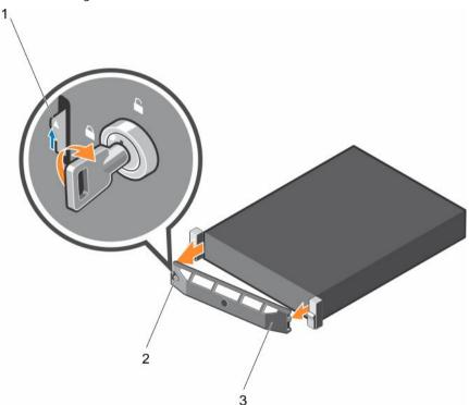
Figure 9. Removing the optional front bezel
