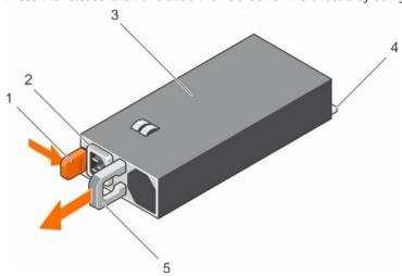
Figure 60. Removing an AC PSU
