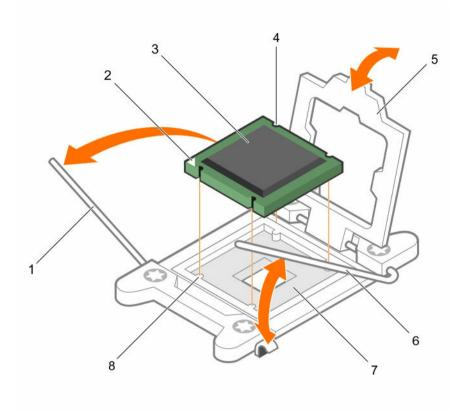
Figure 23. Installing a processor
