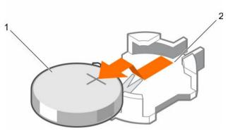
Figure 56. Removing the system battery
