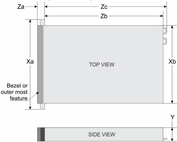
Figure 8. Chassis dimensions of your Dell DR4300 system
