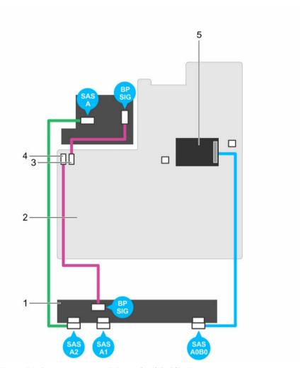
Figure 74. Cabling diagram—3.5 inch (x12) SAS/SATA backplane
