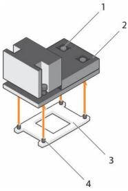
Figure 20. Removing a heat sink
