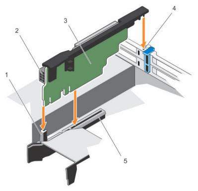
Figure 48. Installing the expansion card riser 3
