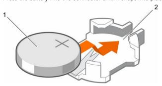
Figure 57. Installing the system battery
