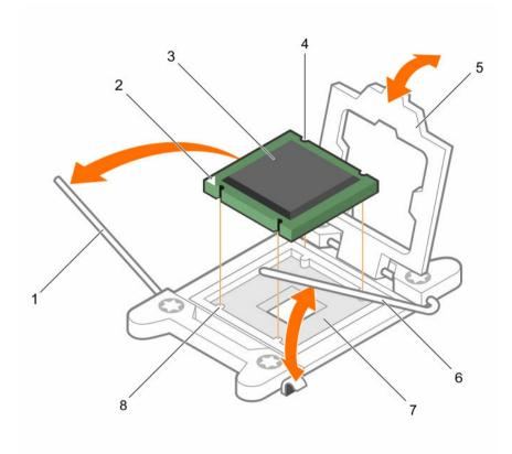
Figure 22. Removing a processor
