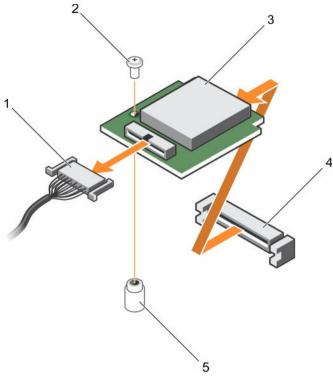
Figure 80. Removing the vFlash media unit
