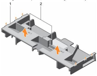
Figure 13. Removing the cooling shroud
