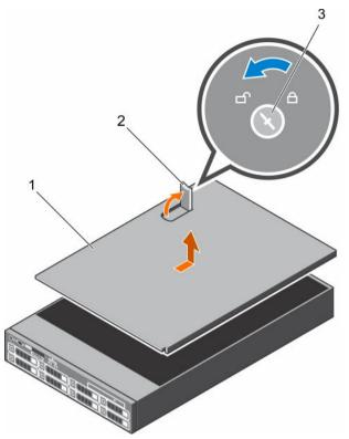
Figure 11. Removing the system cover
