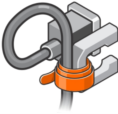
Figure 8. Removing the Hook and Loop Strap from the Power Cable
