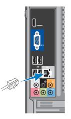
A network connection is not required to complete your computer setup, but if you have an existing network or Internet connection that uses a cable connection (such as a home cable modem or Ethernet jack), you can connect it now. Use only an Ethernet cable (RJ45 connector). Do not plug a telephone cable (RJ11 connector) into the network connector.
