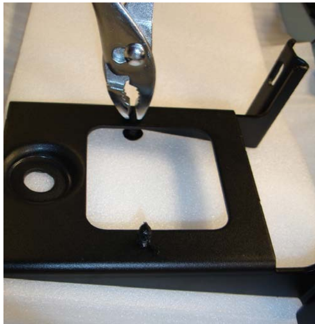
Figure 7: Stabilizer Plastic Fastener Removal
