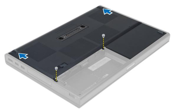
4. Lift and remove the base cover from the computer.
