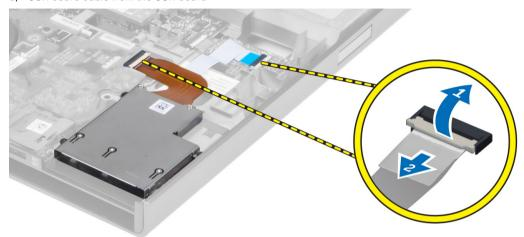
4. Remove the screws that secure the ExpressCard module to the computer and remove the ExpressCard module.
