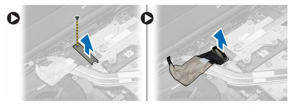
7. Remove the screws that secure the display assembly to the computer. Lift up and remove the display assembly from the computer.
