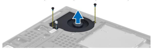
4. Disconnect the processor-fan cable.
