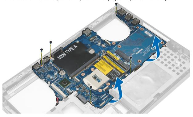
7. Disconnect the power connector cable and remove the system board.
