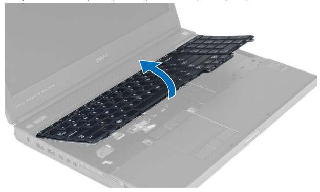
$\textbf{5.} \hspace{0.5cm} \textbf{Disconnect the keyboard-data cable from the system board and remove the keyboard.} \\$
