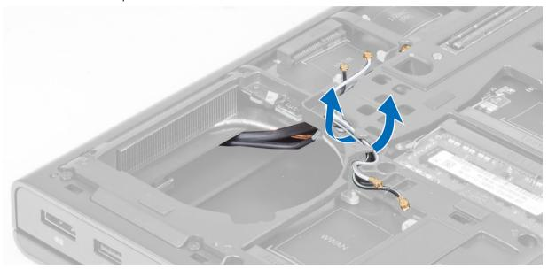
4. Remove the antenna cables from the routing channels.
