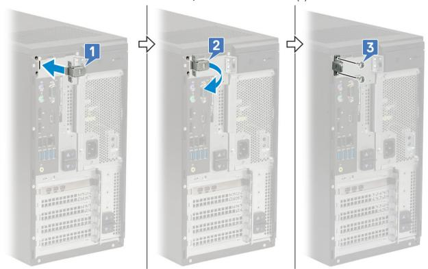
3 Pull the cable release latch and lift the latch away from the cable cover.
