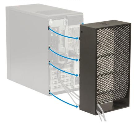
Open the tab and unroute the cables from cable tie [1], disconnect the cables from the ports on the system [2]. Remove the cables from the slot of the cable cover [3].
