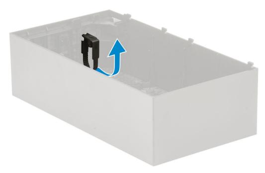
4 Lift the tab [1] to release and pull the cable tie from the slot on the cable release latch [2].
