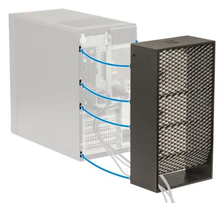
8 Gently press down on the cable cover until it clicks into place [1]. Slide the latch towards the chassis [2] to lock the cable cover in place.
