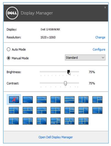
The **Quick Settings** dialog box also provides access to Dell display manager's advanced user interface, which is used to adjust basic functions, configure Auto Mode, and access other features.
