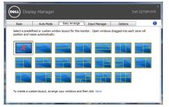
To create a custom window layout, size and position the windows (maximum 10) on the desktop and then click the **Save** link in **Easy Arrange**. The size and position of the windows is saved as a custom layout and the custom layout icon is created.
