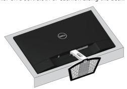
2. Tilt the stand downwards to access to the release button.
