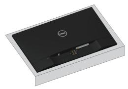
2. Fit the stand riser and stand base together, and then turn the screw in the stand base.
