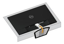
**3.** Use a long screwdriver to press on the release button.
