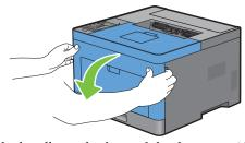
**2** Grasp the handle on the front of the drum cartridge, and then pull it out halfway with one hand.
