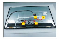
S9 Unplug the LVDS cable from the connector of the panel module by pushing the earing-locks.
