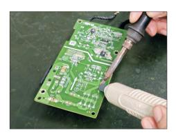
S16-5 Lift the bulk cap. up and away from the PCB.
