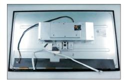
Release the panel module away from the hooks of the front bezel, then lift up the panel module and take away the front bezel with key board.
