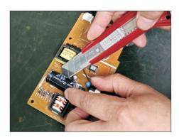
S16-2 Ensure cutting path within the glue, don't touch bulk cap. or PCB.
