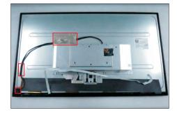
Use a Philips-head screwdriver to remove 2pcs screws for unlocking the bracket with panel module. Use a Hex-head screwdriver to remove 2pcs screws for unlocking the VGA connector.
