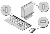
b. Press the wireless sync button at the back of your computer and then the wireless sync button on your keyboard.
