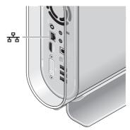
Use only an Ethernet cable (RJ - 45 connector). Do not plug a telephone cable (RJ-11 connector) into the network connector.
