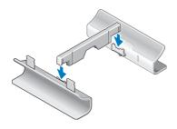
5. Align the securing tabs on the stand with the slots on the computer and lower the computer onto the stand until the securing tabs are inserted into the slots.
