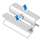
**4.** Turn the stand over and align the stabilizer bar with the securing slots on the stand.
