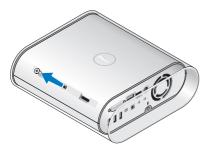
Place the computer vertically and pull the sleeve gently towards the back of your computer, then gently slide the new sleeve onto the computer.
