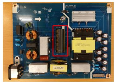
S17-1 Cut the glue between bulk cap. and PCB with a knife
