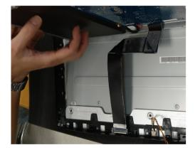
S11 Unlock 14 screws to disassemble Middle Frame
