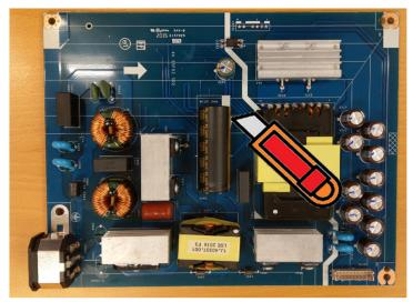
S17-2 Ensure cutting path within the glue, don't touch bulk cap. or PCB
