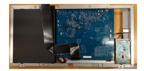
**S15** Unlock 10 PCBA screws to disassemble I/F BD, SPS BD and LED Driver BD from Main SHD
