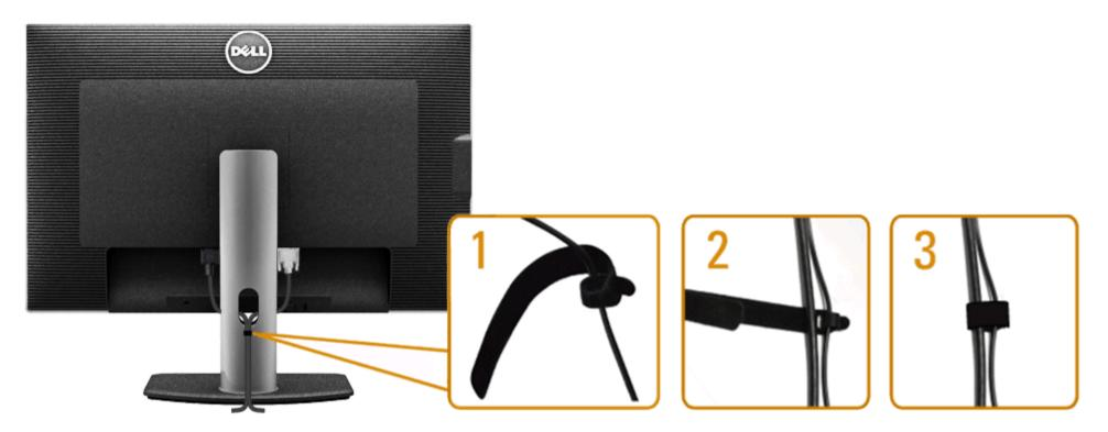
After attaching all necessary cables to your monitor and computer, (See <u>Connecting Your Monitor</u> for cable attachment,) use the Velcro cable tie to organize all cables as shown above.
