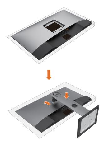
**1** Remove the monitor protective cover and place the monitor with its front facing downward on it.
