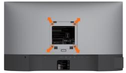
MOTE: Use M4 x 10 mm screws to connect the monitor to the wall-mounting kit.
