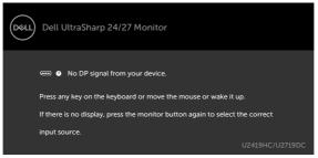
If either DP, USB Type-C input is selected and the corresponding cable is not connected, a floating dialog box as shown below appears.
