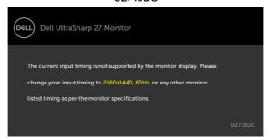
This means that the monitor cannot synchronize with the signal that it is receiving from the computer. See Monitor Specifications for the Horizontal and Vertical frequency ranges addressable by this monitor. Recommended mode is  $1920 \times 1080 \text{ (U2419HC)} / 2560 \times 1440 \text{ (U2719DC)}$ .
