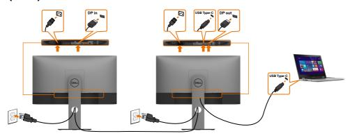
NOTE: The maximum number of supported U2719DC via MST is subjected to the bandwith of the USB-C source. Please refer to "product specific problems –No image when using USB-C MST".
