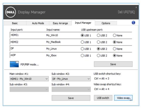
You can assign a USB upstream port with your video input. The assigned USB upstream port will be connected to the computer when its video is showing on the monitor.
