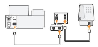
If the additional device (telephone or answering machine) has an RJ-11 connector, then you can remove the wrap plug and plug the device into the printer.
