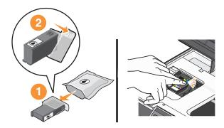
**Note:** Install the ink cartridges immediately after removing the protective cap to avoid exposing the ink to air.
