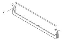
1 securing clip (snapped in position)
