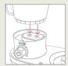
Secure the Coffee Container on the Brewing Base by matching the two circular columns on the underside of the Coffee Container with the corresponding holes in the Brewing Base.
