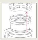
Unscrew and remove the Coffee Container Lid and remove the Brew Basket Assembly.
