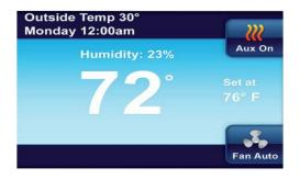
If you have a heat pump, your system will automatically activate Auxiliary Heating when the outside temperature is too cold for the heat pump to efficiently heat your home. When Auxiliary Heating is called for, the display will show "Aux" with the Heat icon
