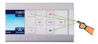
If a voltage spike or static discharge blanks out the display or causes erratic operation of your thermostat, you can reset it.
