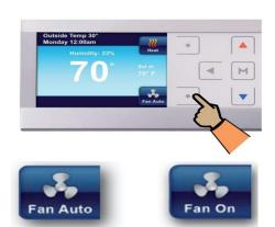
**Fan Auto** This is the most commonly used setting. The fan will turn on only when the heating or cooling system is running.
