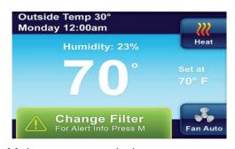
Your thermostat can automatically provide reminders when the air filter, humidifier pad, or UV lamp needs to be replaced. Each of these reminders are turned on or off and the reminder time period set from the appropriate item in the Thermostat Settings Menu (section 3.11).
