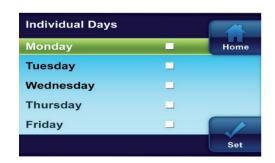
Using **Individual Days** allows you to change the program settings of a single day or days. Highlight a day and press to mark the box. Mark additional days you wish to have programmed the same. Press **Set** to begin entering the program for the selected day or days.
