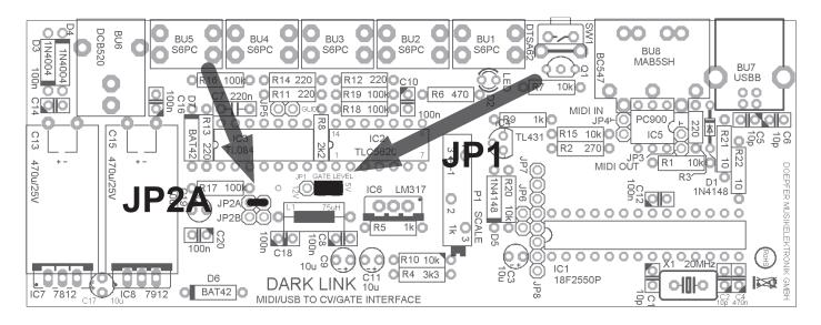
JP1 position for 12 Volts trigger (middle and leftmost contacts)
