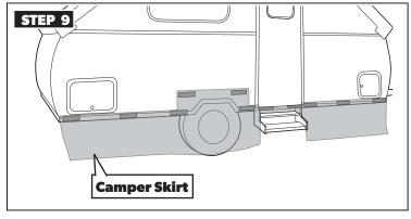
Secure the mesh camper skirt to the Velcro near the wheel well of the camper wall.
