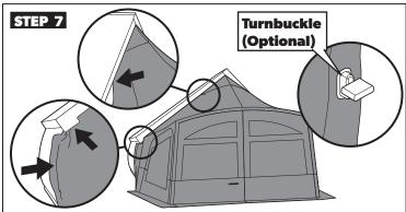
Tuck the Screen Room fabric under the side wall hinge cover on the camper and attach it to the Velcro or turnbuckles on the ends of the camper.
