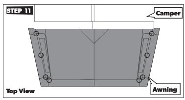
• Stake the inside of the Screen Room to the ground through the loops at the locations shown.
