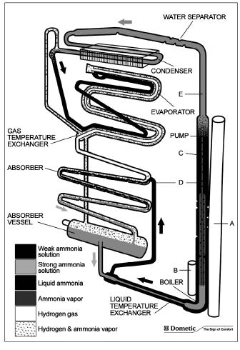
The hydrogen thus circulates continuously between the absorber and the evaporator.
