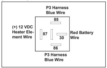
Verify that the following components are good: upper circuit board, thermistor, 5 or 6 wire harness and 30/3-amp fuses. In the DC mode Plug 3, Terminal 4 (positive 86) and Terminal 3 (negative 85) should have voltage to close the relay. If no voltage in the DC mode change the lower board.
