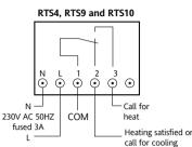
Note: Link between terminals L and 1 if mains voltage is required on the thermostat switch.
