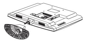
3 Align the base with the bottom of the TV, then secure the base to the TV with the four M5XL 14 mm screws provided.
