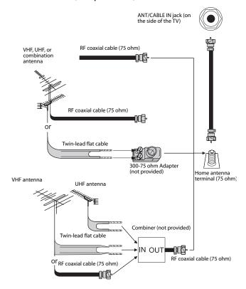
3 Connect the other end of the cable to the **ANT/CABLE IN** jack on the side of your TV.
