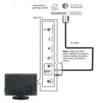
3 Connect the other end of the cable to the AV jack and the AV audio in jacks on the side of your TV.
