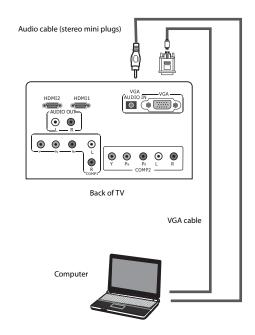
3 Connect an audio cable to the AUDIO OUT jack on the computer, then connect the other end of the cable to the VGA AUDIO IN jack on the back of your TV.
