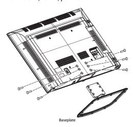
**4** Carefully lift the TV into an upright position. To remove the stand, see the following procedure.
