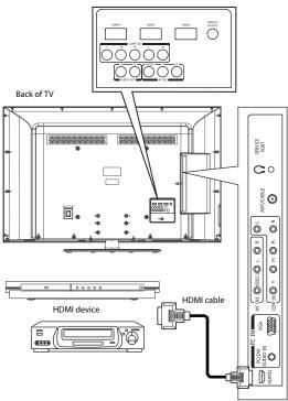
**Note:** To connect a DVI device, use a DVI to HDMI adapter cable to connect to the **HDMI** jack on the TV, then connect an audio cable to the **PC IN AUDIO** jack on the back of the TV.
