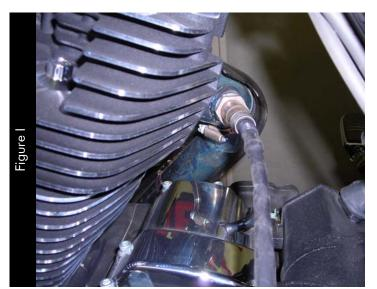
3 Ideally, you should orient the weld boss so the sensor is between the 9 o'clock and 3 o'clock position (reading clockwise) as shown in Figure H. A 10° inclination off the horizontal plane should be considered a minimum.
