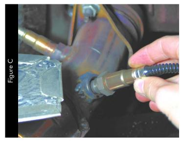
Ideally, you should orient the weld boss so the 3 sensor is between the 9 o'clock and 3 o'clock position (reading clockwise) as shown in Figure B. A 10° inclination off the horizontal plane should be considered a minimum.
