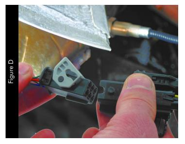
2 Connect the O2 Sensor to the supplied wiring harness as shown in Figure D.
