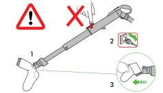
Switch 'OFF' and unplug the appliance before clearing brush bar obstructions.
