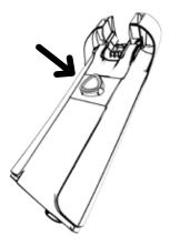
5. Fill remaining Clean Water Solution Tank with hot tap water. Tightly screw cap back on.
