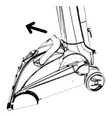
2. Hold the handle and pull tank up and out.
