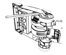
3. With belt in place, pull and slide brushroll into the nozzle, making sure that the brushroll ends are in the correct orientation (A).
