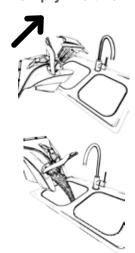
4. Rinse the tank and filter with hot tap water. Wipe and let dry before storing to prevent mildew. Replace the dirty water tank lid.
