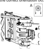
Replace belt cover and secure with the three screws.
