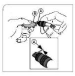
Check the gap (A) with a wire gauge (B). If necessary, reset the gap. Install and tighten the spark plug to the recommended torque. For gap setting or torque, see the **Specifications** section.
