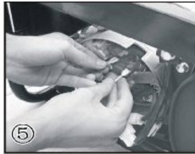
⑤ Insert and connect the DC wire of excitation according to anode-cathode.
