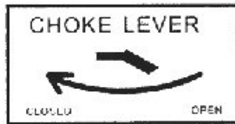
Figure 7- Choke in the “closed” position (refer to choke location)
