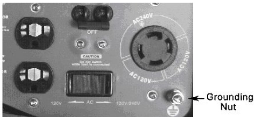
Figure 5 – Attaching the Grounding Wire to the Generator
