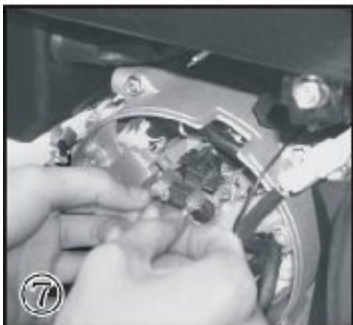
⑦ Insert and connect the DC wire of excitation according to anode-cathode.
