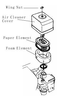
Air Cleaner and Filter Cartridge (Call Lifan Power USA for replacement air filter cartridge's or visit your retailer)
