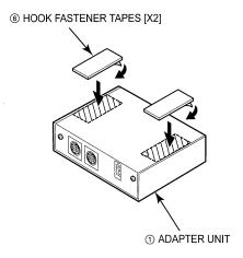
2 Attach the loop fastener tapes to the floor and attach the iPod adapter unit.
