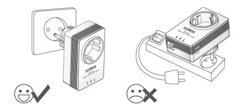
2. If you need to use a multiple socket for additional network devices, then connect the multiple socket to the integrated power socket of the adapter, and plug the powerline directly into a power socket, as shown below. The power socket of the adapter features a filter function which is able to improve the data transmission in the network.
