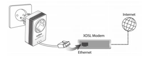
2. Plug another Powerline adapter (HP-5101Wn) into a power socket, and confirm the power LED is on.
