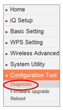
Using the diagnosis tool, you can ping a specific IP address and automatically reboot the device if there is no response.
