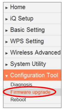
The wireless extender's firmware upgrade feature allows you to upgrade the system firmware to a more recent version. You can download the latest firmware from the Edimax website.
