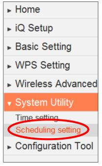
The wireless extender includes a scheduling function, where power saving functions and an automatic reboot can be automated for specific times. By default, scheduling setting is disabled. Please select "Enable" if you wish to continue.
