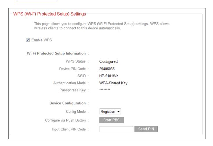
The wireless extender supports two types of WPS for wireless clients: PBC (Push Button Configuration) and PIN code. For PBC you can activate WPS on the wireless extender by clicking the "Start PBC" button on the screen.
