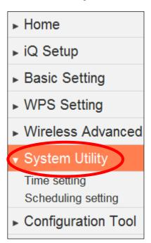
In "System Utility" you can configure the extender's administrative password and manage the extender's IP and DHCP settings.
