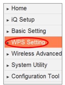
WPS (Wi-Fi Protected Setup) is a simple way to establish connections between WPS compatible devices. WPS devices feature a WPS function which can be activated by pushing a WPS button on the device or from within the device's firmware/configuration interface. When WPS is activated in the correct manner and at the correct time for two compatible devices, they will automatically connect.
