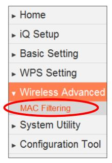
The MAC filtering feature allows you to define a list of wireless devices permitted to connect to this access point, identified by their unique MAC address. When a device which is not listed as a permitted MAC address attempts to connect to the extender, it will be denied.
