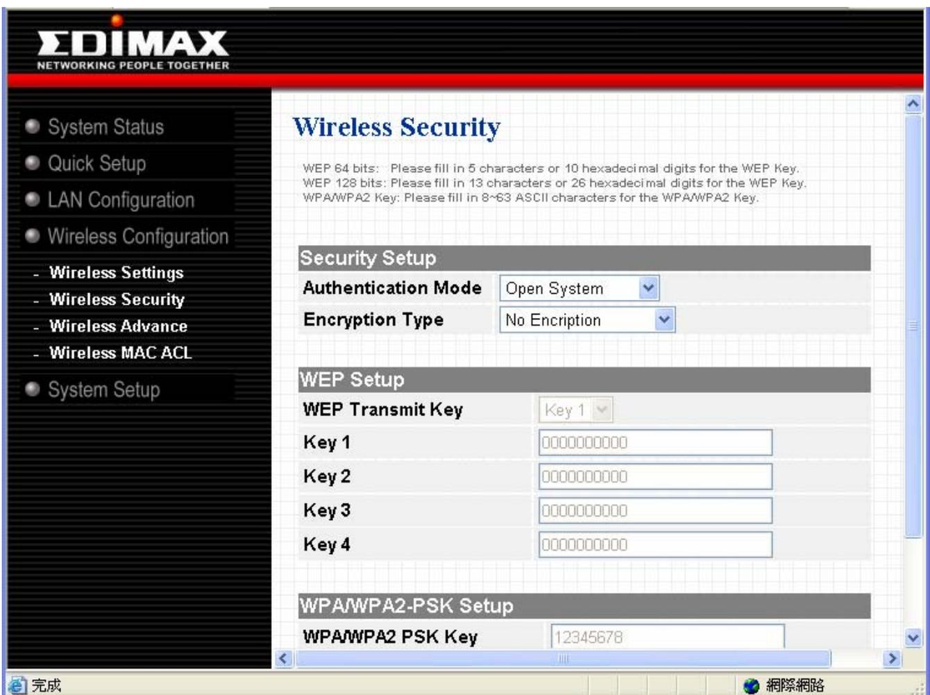
The Authentication type supports "Open system", "Shared key", "WPA-PSK", "WPA2-PSK" and "WPA-PSK/WPA2-PSK".
